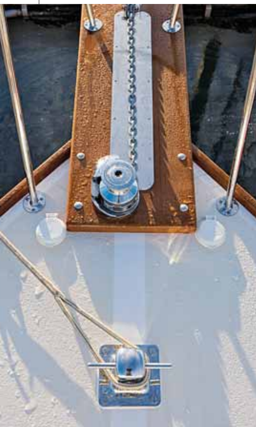
The forward deck of the 34 features nonskid that’s effective even when wet, as well as beefy stainless hardware. Note the chafing plate for the anchor chain.
