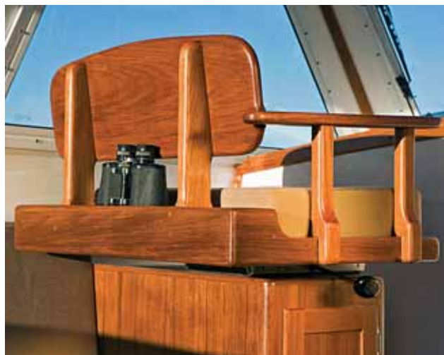
The custom-built, teak helm and companion seats (above) slide back and forth, and they sit atop sturdy, matching storage cabinets.
